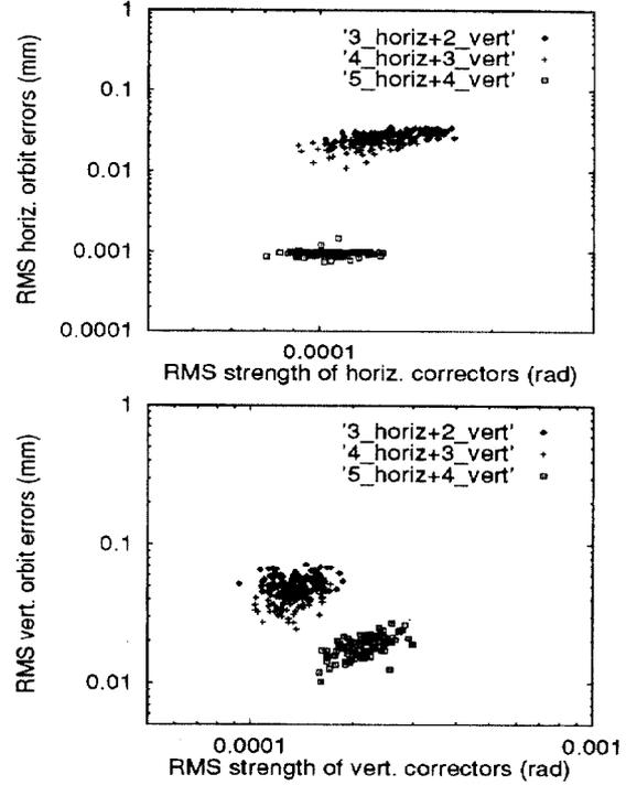
Figure 4: Resulting closed orbit error as a function of different numbers of correctors.
