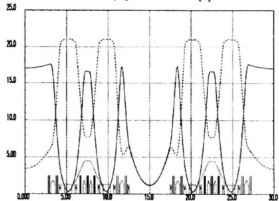
Figure 1: Linear lattice functions of the BESSY II cell.
