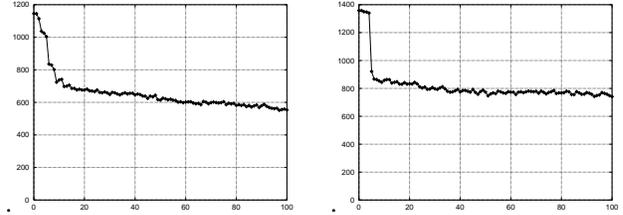
Figure 1: A fast beam loss onto the dynamic (left) and physical (right) aperture. The first 100 revolutions are shown.
